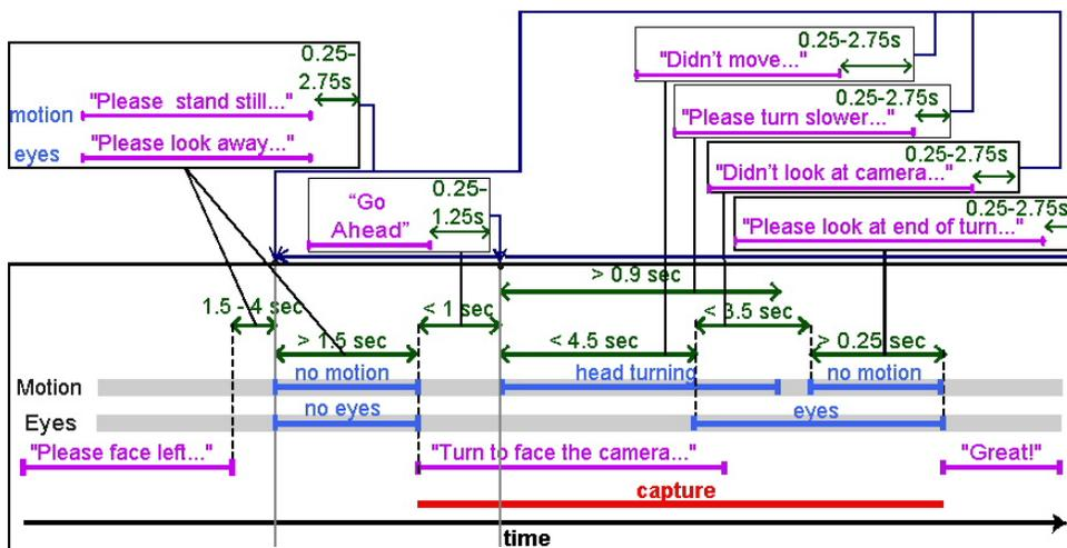
**Figure 2. Visualization of "Head Turn" Active Capture scenario. The application directs the guest to turn her head to look at the camera by ensuring a set of constraints are satisfied through a control process with interactive feedback**
